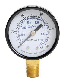
ProSense mechanical pressure gauge, 2in diameter, 0 to 100 psig/0 to 700 kPa, black steel dry case, brass wetted parts, 1/4in male NPT process connection, lower mount.
