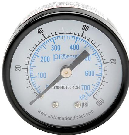
ProSense mechanical pressure gauge, 2in diameter, 0 to 100 psig/0 to 700 kPa, black steel dry case, brass wetted parts, 1/4in male NPT process connection, center back mount.
