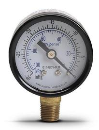
ProSense mechanical pressure gauge, 1.5in diameter, -30 to 0in Hg vacuum/-100 to 0 kPa, black steel dry case, brass wetted parts, 1/8in male NPT process connection, lower mount.
