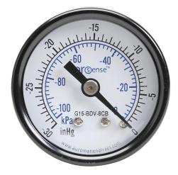
ProSense mechanical pressure gauge, 1.5in diameter, -30 to 0in Hg vacuum/-100 to 0 kPa, black steel dry case, brass wetted parts, 1/8in male NPT process connection, center back mount.
