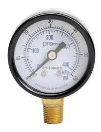
ProSense mechanical pressure gauge, 1.5in diameter, 0 to 60 psig/0 to 400 kPa, black steel dry case, brass wetted parts, 1/8in male NPT process connection, lower mount.
