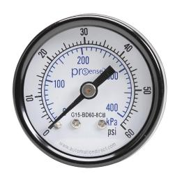
ProSense mechanical pressure gauge, 1.5in diameter, 0 to 60 psig/0 to 400 kPa, black steel dry case, brass wetted parts, 1/8in male NPT process connection, center back mount.
