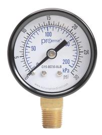
ProSense mechanical pressure gauge, 1.5in diameter, 0 to 30 psig/0 to 200 kPa, black steel dry case, brass wetted parts, 1/8in male NPT process connection, lower mount.
