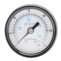
ProSense mechanical pressure gauge, 1.5in diameter, 0 to 30 psig/0 to 200 kPa, black steel dry case, brass wetted parts, 1/8in male NPT process connection, center back mount.
