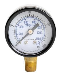
ProSense mechanical pressure gauge, 1.5in diameter, 0 to 200 psig/0 to 1400 kPa, black steel dry case, brass wetted parts, 1/8in male NPT process connection, lower mount.
