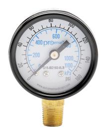
ProSense mechanical pressure gauge, 1.5in diameter, 0 to 160 psig/0 to 1100 kPa, black steel dry case, brass wetted parts, 1/8in male NPT process connection, lower mount.
