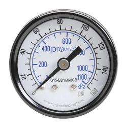
ProSense mechanical pressure gauge, 1.5in diameter, 0 to 160 psig/0 to 1100 kPa, black steel dry case, brass wetted parts, 1/8in male NPT process connection, center back mount.
