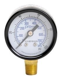
ProSense mechanical pressure gauge, 1.5in diameter, 0 to 100 psig/0 to 700 kPa, black steel dry case, brass wetted parts, 1/8in male NPT process connection, lower mount.
