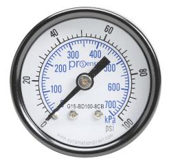
ProSense mechanical pressure gauge, 1.5in diameter, 0 to 100 psig/0 to 700 kPa, black steel dry case, brass wetted parts, 1/8in male NPT process connection, center back mount.
