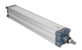
NITRA pneumatic cylinder, ISO 15552, 100mm bore, 25mm rod diameter, 600mm stroke, double acting, magnetic piston, front and rear adjustable cushions.
