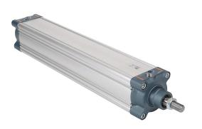
NITRA pneumatic cylinder, ISO 15552, 100mm bore, 25mm rod diameter, 500mm stroke, double acting, magnetic piston, front and rear adjustable cushions.
