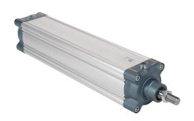
NITRA pneumatic cylinder, ISO 15552, 100mm bore, 25mm rod diameter, 400mm stroke, double acting, magnetic piston, front and rear adjustable cushions.
