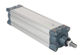
NITRA pneumatic cylinder, ISO 15552, 100mm bore, 25mm rod diameter, 300mm stroke, double acting, magnetic piston, front and rear adjustable cushions.
