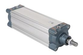
NITRA pneumatic cylinder, ISO 15552, 100mm bore, 25mm rod diameter, 250mm stroke, double acting, magnetic piston, front and rear adjustable cushions.
