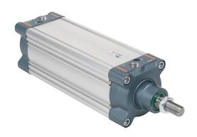
NITRA pneumatic cylinder, ISO 15552, 100mm bore, 25mm rod diameter, 200mm stroke, double acting, magnetic piston, front and rear adjustable cushions.
