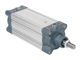
NITRA pneumatic cylinder, ISO 15552, 100mm bore, 25mm rod diameter, 150mm stroke, double acting, magnetic piston, front and rear adjustable cushions.
