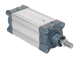
NITRA pneumatic cylinder, ISO 15552, 100mm bore, 25mm rod diameter, 125mm stroke, double acting, magnetic piston, front and rear adjustable cushions.
