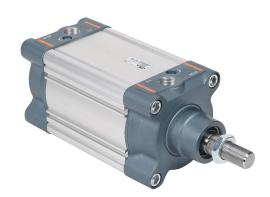
NITRA pneumatic cylinder, ISO 15552, 100mm bore, 25mm rod diameter, 75mm stroke, double acting, magnetic piston, front and rear adjustable cushions.
