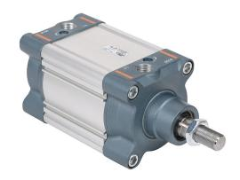
NITRA pneumatic cylinder, ISO 15552, 100mm bore, 25mm rod diameter, 50mm stroke, double acting, magnetic piston, front and rear adjustable cushions.
