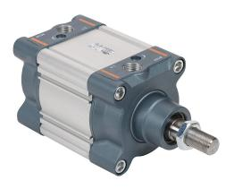
NITRA pneumatic cylinder, ISO 15552, 100mm bore, 25mm rod diameter, 25mm stroke, double acting, magnetic piston, front and rear adjustable cushions.
