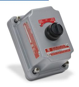
Killark control station cover assembly, hazardous location rated, factory sealed, single selector switch, knob, 3-position, black, spring return to center from left, maintained center and right, (2) N.O. contact(s), legend plate marking "HAND OFF AUTO".
