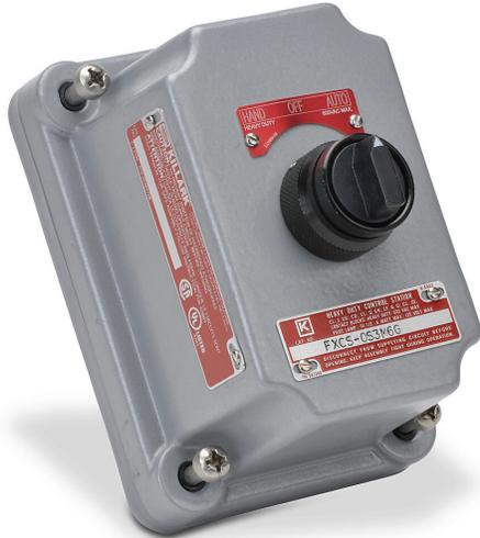
Killark control station cover assembly, hazardous location rated, factory sealed, single selector switch, knob, 3-position, black, spring return to center from right or left, (2) N.O. contact(s), legend plate marking "HAND OFF AUTO".
