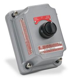
Killark control station cover assembly, hazardous location rated, factory sealed, single selector switch, knob, 3-position, black, spring return to center from right, maintained center and left, (2) N.O. contact(s), legend plate marking "HAND OFF AUTO".
