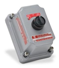
Killark control station cover assembly, hazardous location rated, factory sealed, single selector switch, knob, 3-position, black, maintained, (2) N.O./(2) N.C. contact(s), legend plate marking "HAND OFF AUTO".
