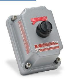
Killark control station cover assembly, hazardous location rated, factory sealed, single selector switch, knob, 3-position, black, maintained, (1) N.O./(1) N.C. contact(s), legend plate marking "HAND OFF AUTO".
