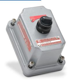
Killark control station cover assembly, hazardous location rated, factory sealed, single selector switch, knob, 2-position, black, spring return from right, (1) N.O./(1) N.C. contact(s), legend plate marking "OFF ON".
