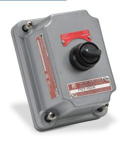
Killark control station cover assembly, hazardous location rated, factory sealed, single selector switch, knob, 2-position, black, maintained, (2) N.O./(2) N.C. contact(s), legend plate marking "OFF ON".
