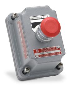
Killark control station cover assembly, hazardous location rated, factory sealed, single pushbutton, mushroom, red, push-pull, (1) N.O./(1) N.C. contact(s), (3) two-sided legend plate(s), legend plate marking "START,STOP / EMERGENCY STOP, RESET / blank, RESET".
