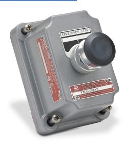
Killark control station cover assembly, hazardous location rated, factory sealed, single pushbutton, mushroom, black, push-pull, (1) N.O./(1) N.C. contact(s), legend plate marking "START,STOP / EMERGENCY STOP, RESET / blank, RESET".
