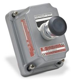
Killark control station cover assembly, hazardous location rated, factory sealed, single pushbutton, mushroom, black, push-pull, (1) N.O./(1) N.C. contact(s), legend plate marking "START,STOP / EMERGENCY STOP, RESET / blank, RESET".
