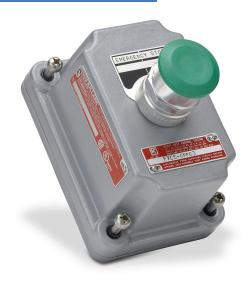
Killark control station cover assembly, hazardous location rated, factory sealed, single pushbutton, mushroom, green, push-pull, (1) N.O./(1) N.C. contact(s), (3) two-sided legend plate(s), legend plate marking "START,STOP / EMERGENCY STOP, RESET / blank, RESET".
