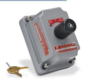
Killark control station cover assembly, hazardous location rated, factory sealed, single selector switch, key-operated, 3-position, black, spring return to center from left, maintained center and right, (2) N.O. contact(s), legend plate marking "HAND OFF AUTO".
