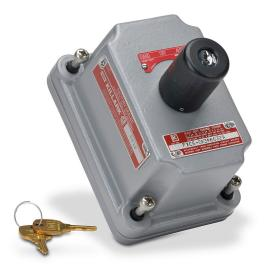
Killark control station cover assembly, hazardous location rated, factory sealed, single selector switch, key-operated, 3-position, black, spring return to center from right or left, (2) N.O. contact(s), legend plate marking "HAND OFF AUTO".
