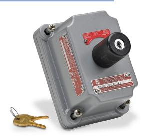
Killark control station cover assembly, hazardous location rated, factory sealed, single selector switch, key-operated, 3-position, black, spring return to center from right, maintained center and left, (2) N.O. contact(s), legend plate marking "HAND OFF AUTO".
