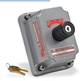
Killark control station cover assembly, hazardous location rated, factory sealed, single selector switch, key-operated, 3-position, black, maintained, (2) N.O./(2) N.C. contact(s), legend plate marking "HAND OFF AUTO".
