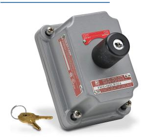
Killark control station cover assembly, hazardous location rated, factory sealed, single selector switch, key-operated, 2-position, black, spring return from right, (1) N.O./(1) N.C. contact(s), legend plate marking "OFF ON".
