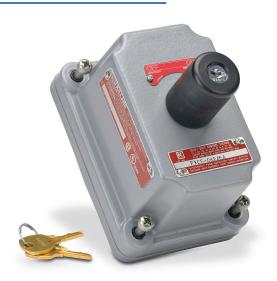
Killark control station cover assembly, hazardous location rated, factory sealed, single selector switch, key-operated, 2-position, black, maintained, (2) N.O./(2) N.C. contact(s), legend plate marking "OFF ON".
