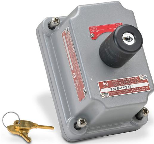
Killark control station cover assembly, hazardous location rated, factory sealed, single selector switch, key-operated, 2-position, black, maintained, (1) N.O. and (1) N.C. contact(s), legend plate marking "OFF ON".
