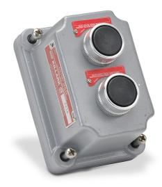
Killark control station cover assembly, hazardous location rated, factory sealed, two pushbuttons, black/black, momentary, (1) N.O/ (1) N.C. and (1) N.O/(1) N.C. contact(s), (2) blank legend plate(s).
