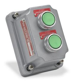
Killark control station cover assembly, hazardous location rated, factory sealed, two pushbuttons, green/green, momentary, (1) N.O. and (1) N.O. contact(s), legend plate marking "START / START".
