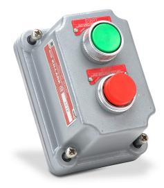
Killark control station cover assembly, hazardous location rated, factory sealed, two pushbuttons, red/green, momentary, (1) N.O. and (1) N.C. contact(s), legend plate marking "START / STOP".
