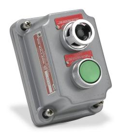
Killark control station cover assembly, hazardous location rated, factory sealed, single pilot light, single pushbutton, green, 110 VAC/VDC LED, green, momentary, (1) N.O. contact(s), blank legend plate(s), legend plate marking "START".
