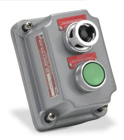
Killark control station cover assembly, hazardous location rated, factory sealed, single pilot light, single pushbutton, green, 110 VAC/VDC LED, green, momentary, (1) N.O. contact(s), blank legend plate(s), legend plate marking "START".
