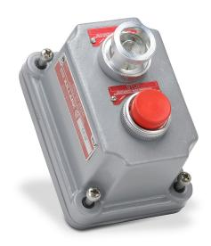
Killark control station cover assembly, hazardous location rated, factory sealed, single pilot light, single pushbutton, red, 110 VAC/VDC LED, clear/white, momentary, (1) N.C. contact(s), blank legend plate(s), legend plate marking "STOP".
