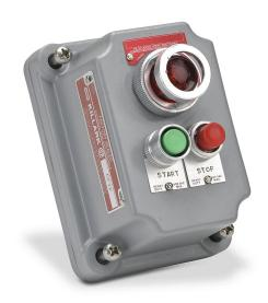
Killark control station cover assembly, hazardous location rated, factory sealed, single pilot light, two mini-pushbuttons, red/green, 110 VAC/VDC LED, red, momentary, (1) N.O./(1) N.C. contact(s), blank legend plate(s), legend plate marking "START, STOP".
