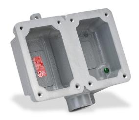
Killark device/splice box, dead end, (2) gang, factory sealed, (1) 1in female NPT conduit entries, aluminum. Use with FXCS series factory sealed cover assemblies for hazardous locations.
