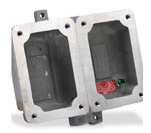
Killark device/splice box, dead end, (2) gang, factory sealed, (1) 3/4in female NPT conduit entries, aluminum. Use with FXCS series factory sealed cover assemblies for hazardous locations.
