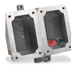
Killark device/splice box, dead end, (2) gang, factory sealed, (1) 3/4in female NPT conduit entries, aluminum. Use with FXCS series factory sealed cover assemblies for hazardous locations.
