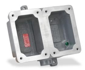
Killark device/splice box, dead end, (2) gang, factory sealed, (1) 1/2in female NPT conduit entries, aluminum. Use with FXCS series factory sealed cover assemblies for hazardous locations.
